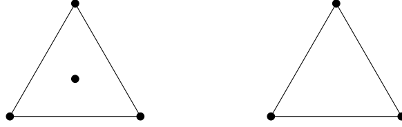
Figure 7.10: The \mathbb{P}_1 -bubble/ \mathbb{P}_1 (mini) element for velocity (left) and pressure (right) approximation.
