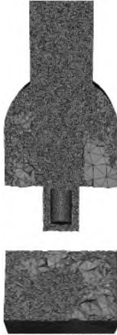
Fig. 5. Adapted meshes: cut through the tetrahedral mesh.
