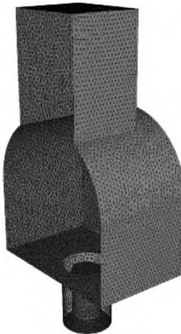
Fig. 2. Computational mesh: mesh generated by YAMS.
