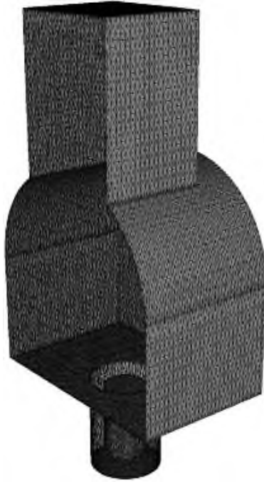
Fig. 1. Mesh generated by FreeFEM3d.
