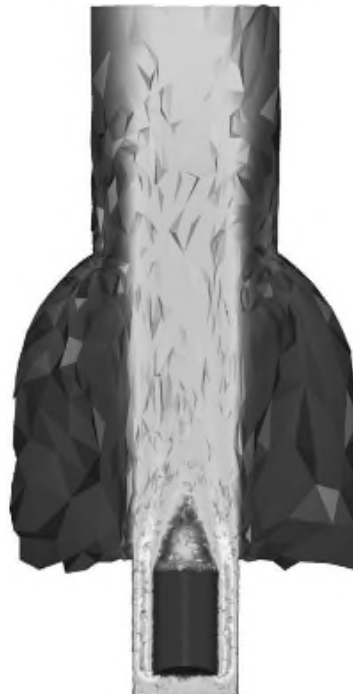
Fig. 8. Adapted meshes: cut through the tetrahedra and associated velocity field (on the top).
