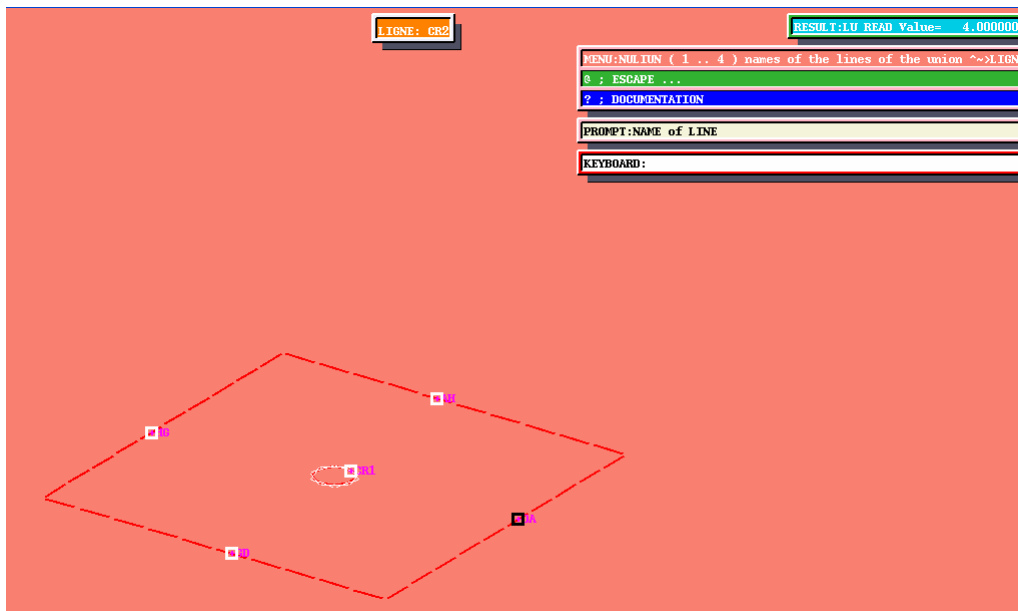
Figure 38: we use mouse to select 4 lines., click 4 smaller rectangles on red line
